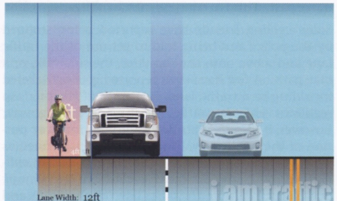
On this illegal pass, the shadow bar surrounding the cyclist represents the required minimum three-foot passing cushion off the right side of the truck (graphic courtesy of IAmTraffic.org and Keri Caffrey)
